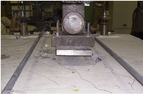
Fig. 4. Punching shear failure of the restrained deck test.
